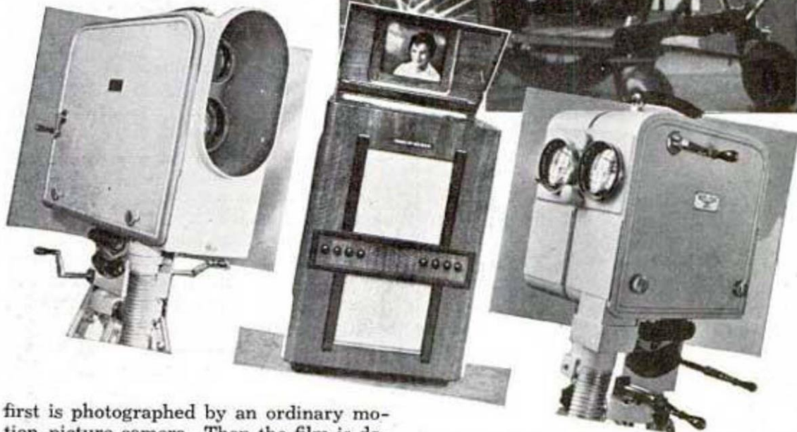
Top, how television pictures are taken. Bottom, left, electron-tube camera for use in stage work. Center, receiver with nineteen-inch cathode-ray tube. Right, small, easily portable television camera for indoor and outdoor work
