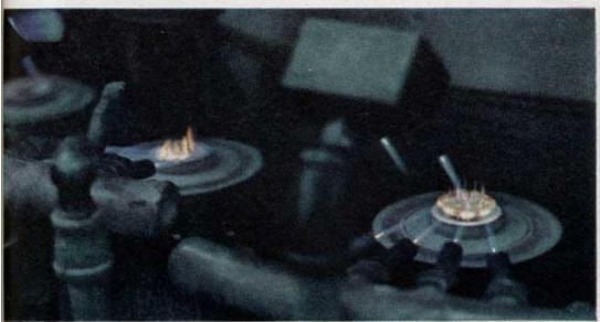
Automatic burners seal a glass ring to the head wire, on which the electrodes are mounted. After the stem is sealed to the bulb, it will be ready for the vacuum pumps. A big problem in designing this mass-production system for cathode-ray tubes was cleanliness. No machine could be permitted to stir up dust, leak oil or
