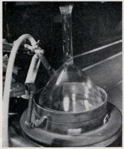
The empty bulb that will become a television picture tube is preheated on a 16-head rotary machine, as shown above, before the metal button for the second anode is inserted in its side. The button is made of a special alloy that conducts electricity well and also forms a vacuumtight weld with glass wall of the tube.
