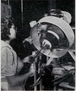
Following application of the phosphor coating, which glows to produce the television picture, the inside of a tube is swabbed with a mixture of graphite and silver that forms a conducting surface. This machine rotates the bulb while the operator holds the swab inside. Later a similar coat is applied to the outside.
