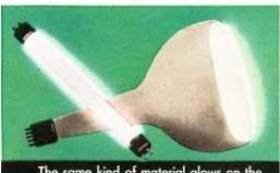
The same kind of material glows on the walls of a fluorescent lamp as on the face of a picture tube.
