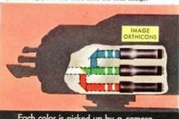
Each color is picked up by a camera picture tube called an image orthicon.
