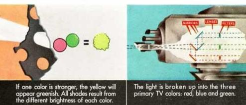
9 GLOWING COLORED DOTS on the screen, too tiny to be seen by the human eye, tuse and blend together, like the dots in these color engravings, to produce the right color.
