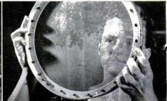
6 ASSEMBLY OPERATION is next. RCA operator holds shadow mask. Unlike one-piece black-and-white tubes, color tubes have a separate conical body and tube face. Present costly handwork will be mechanized later.
