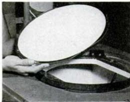
5 DRIED, PHOSPHOR-COATED tube face is put over light source for study under microscope for any flaws in servings of red, green and blue phosphors. Colors are due to addition of silver or copper activals rs to phosphors.
