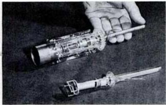
7 ELECTRON COLOR GUN—actually three guns in one—is bigger than that for black-andwhite TV, in foreground. RCA has demonstrated experimental tubes bigger than present developmental types.
