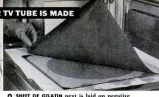
2 SHEET OF GELATIN next is laid on negative plate. Exposed to ultraviolet light, it hardens except where 200,000 tiny dots on negative obstruct the light. Soft gelatin behind the dots is dissolved out with water, leaving a stencil for phosphoring the tube face.
