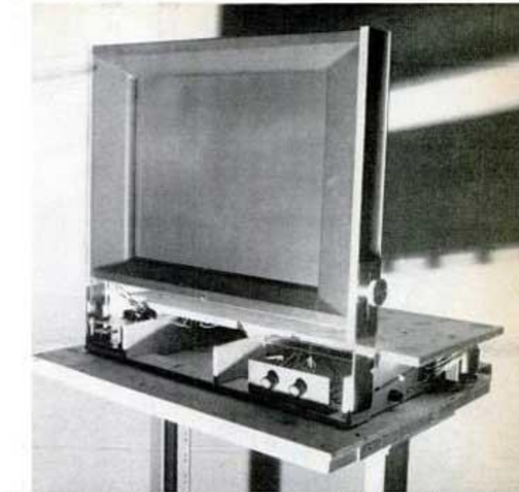
Slim rectangular frame of converter is a bit larger than viewing area. A simple adapter plug snaps onto picture-tube pins, feeding in color signals from circuit in converter
