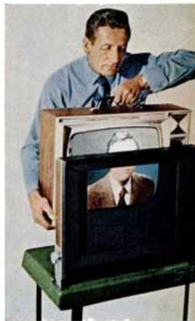
Slide your black-and-white set behind this moving-belt converter and you see a color picture. Picture tube needs adapter plug.
