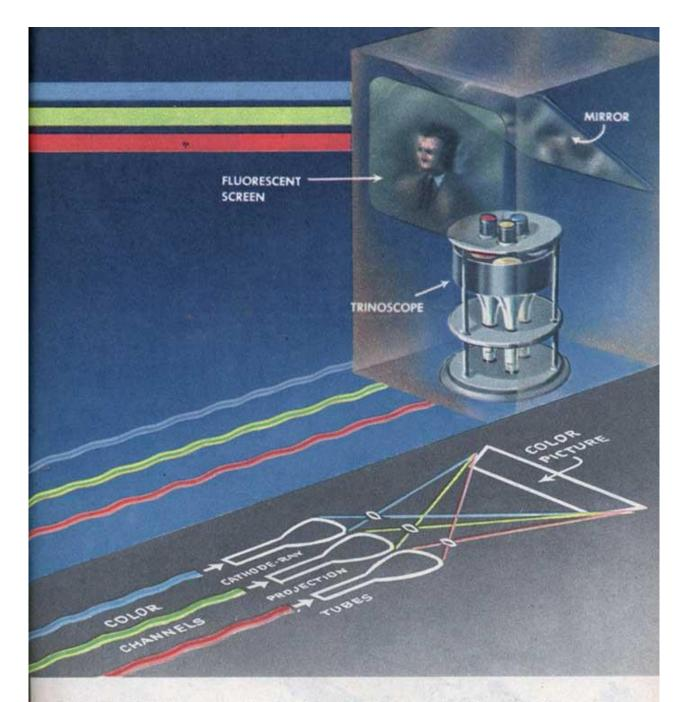
A LL-ELECTRONIC color television, a which RCA engineers have achieved in a form that does not make black-andwhite equipment obsolete, is a complete departure from the mechanical color transmissions of recent years. Mirrors and photoelectric cells replace moving parts.
