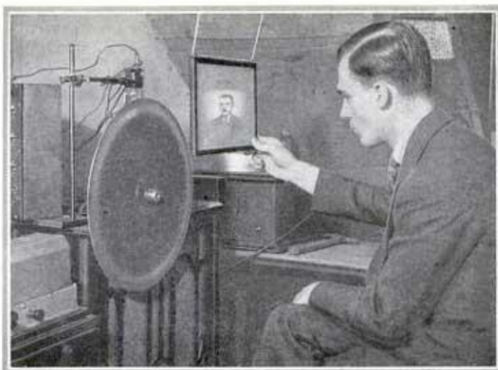
Fig. 1. The author operating a lens disk receiver. Above: How parts are arranged
