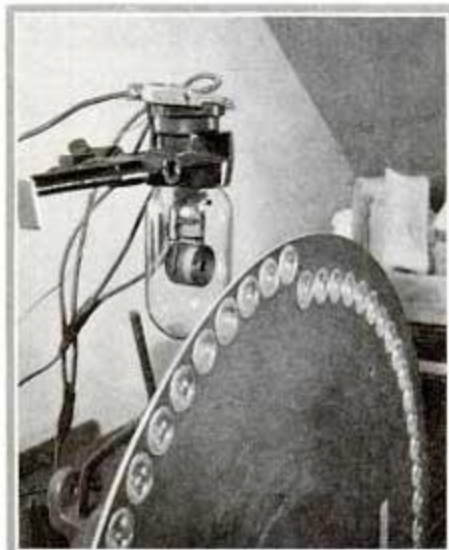
Fig. 4. Detail showing the crater neon lamp and the top of the spiral of tiny lenses. The disk rotates clockwise
