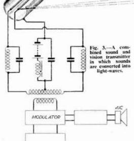
proportional to the original voice frequencies. Now when these side-band voltages are applied to the rod electrodes, the actual spark is found to "prefer" to discharge itself, at the particular point along the coil which is "in tune " with its own frequency.
