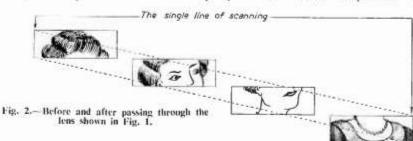
verts the usual square or rectangular surface into a new shape, which has the same light-and-shade values as the original picture, but is "spread out" into a single line. By transforming the picture from a two-dimensional to a one-dimensional form—without having to use any moving parts—the subsequent operation of scanning is greatly simplified.
