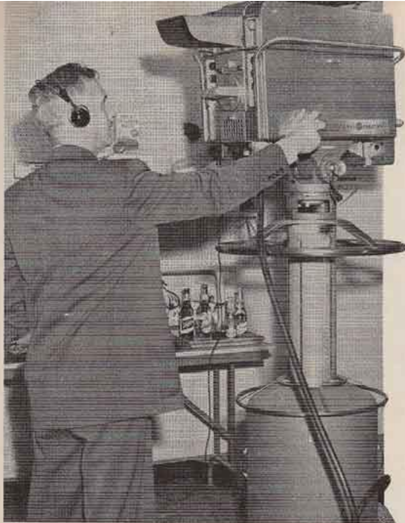
A conventional monochrome TV camera which has been modified for color operation is being adjusted for a studio color shot.
