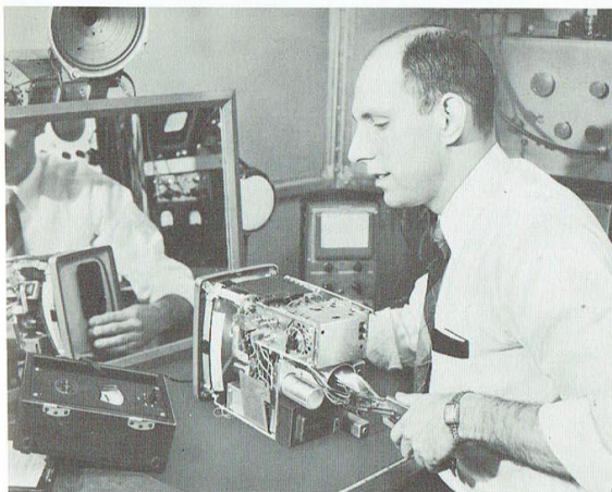
Fig. 5—G. E. Skorup measuring light output versus ion-trap magnet adjustment. Notice the special tool for adjusting the ion-trap inside the kinescope neck shield.
