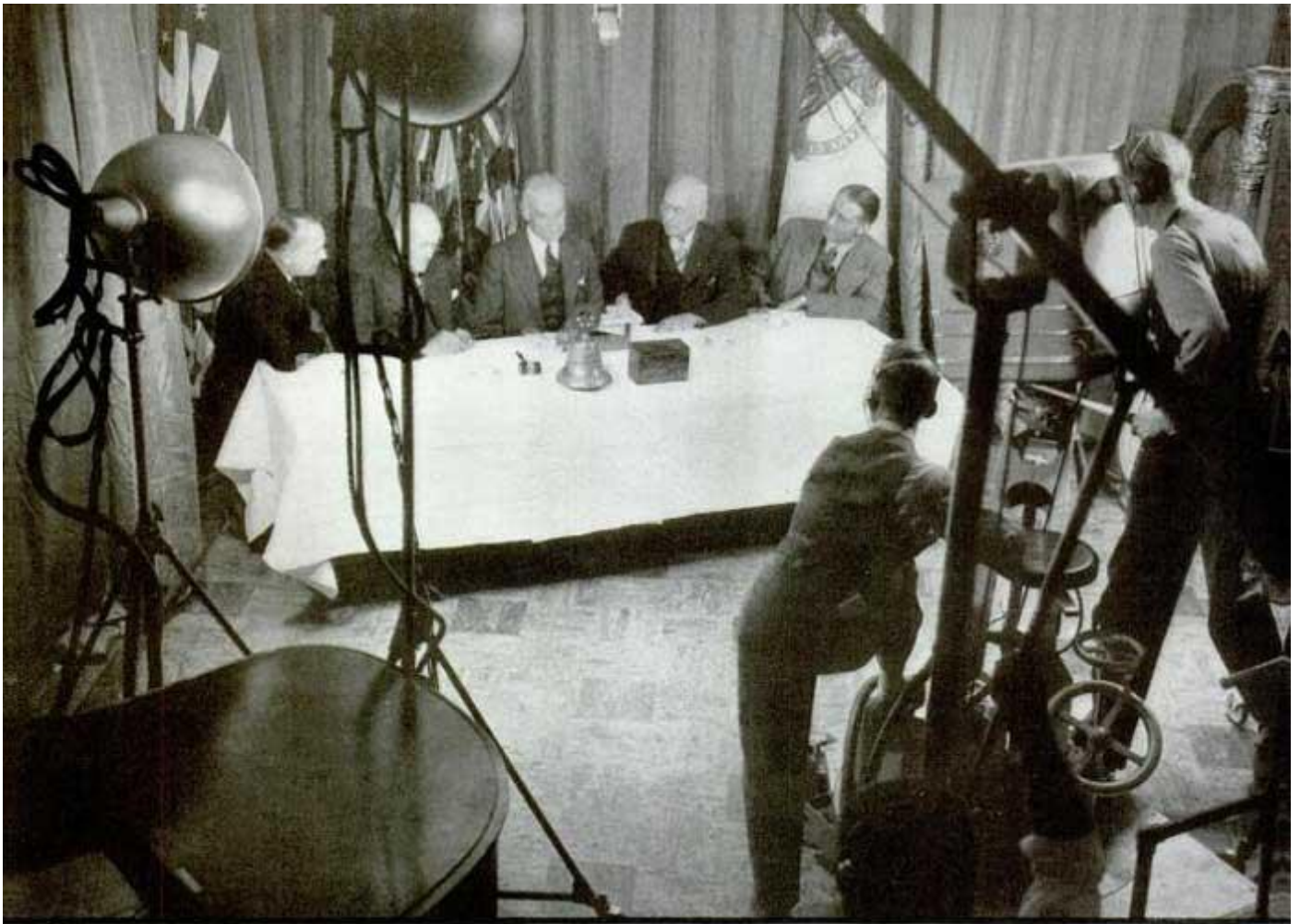
THE telecast originated in this studio (above), a pleasant jungle of cables and water-cooled lights. Heart of the room is the "dolly" which carries the camera (the streamlined box through which the operator peers stereoscopically) and the microphone. At the "speakers' table" are (left to right) Schenectady Rotarian Carl W. Snyder, the general chairman, Founder Harris, President Head, Secretary Perry, and Leland D. Case, The Rotarian editor. District Governor Charles S. Morris, not shown in picture, also took part.
