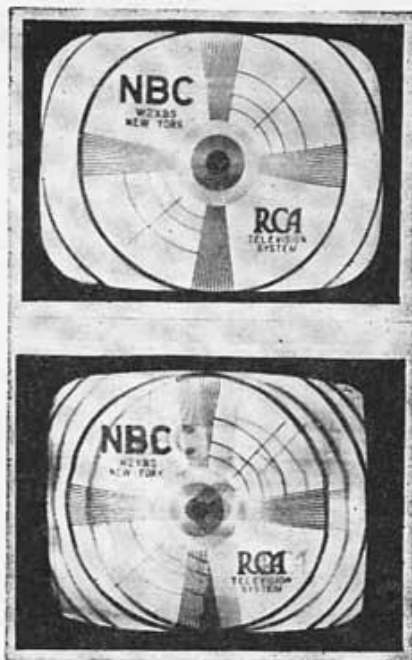
Top—Fig. 2, shows normal "test pattern." Lower photo—Fig. 3, shows "test pattern" marred by a reflected or multi-path signal.
