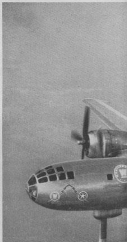
The experimental Stratovision station (a modified B-29), flying at 25,000 feet over the Pittsburgh area, rebroadcast telecast picked up from the east coast television network over an estimated area 525 miles in diameter. Programs from the ground stations are picked up on the antenna projecting above the tail, and rebroadcast from the long, mast-like antenna extending down from the nose of the plane.
