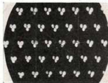
Fig. 8. The pattern appearing on the face of a color tube when a dot generator is used and the d.c. convergence voltage is lower than normally required.
