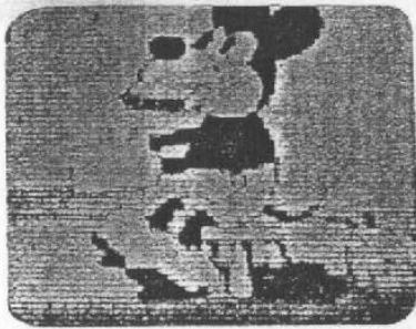
FIG. 7A The 60-line scanning of the early mechanical systems yielded a result like this. The subject is a Mickey Mouse cartoon.
