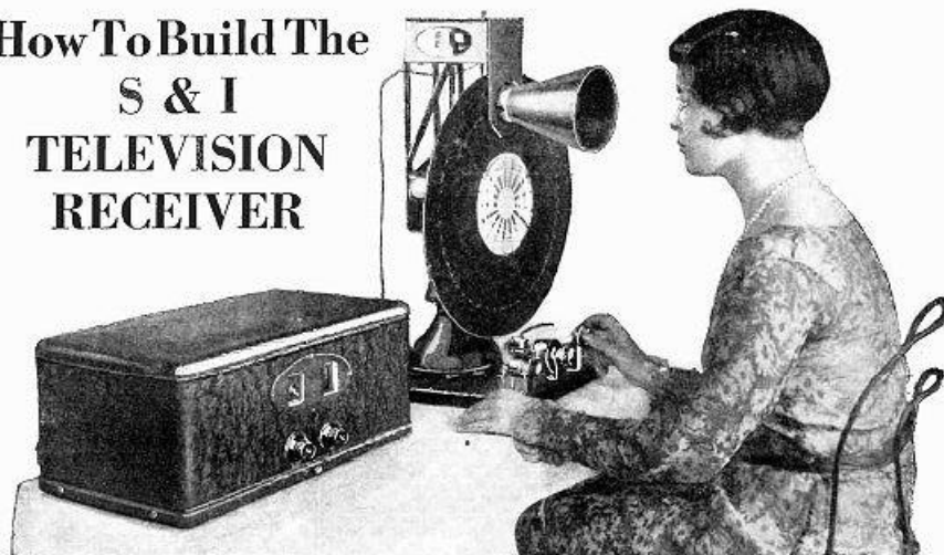
A slight adjustment of the rheostats and the picture comes in clearly. This photo shows a complete television receiver connected to an ordinary radio set. The picture is seen in the case.
