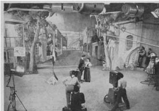
*A glimpse into a modern television studio during the televising of a playlet. Amid a realistic stage setting, note the two television cameras, the microphone hung on its long overhead arm, and the powerful lights.*
