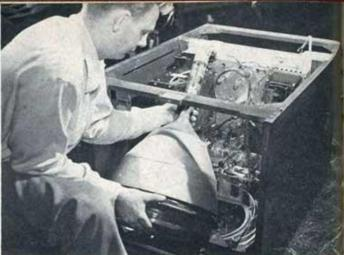
A Tri-color tube is easily installed by laying cabinet face down on floor, with top removed. μ-metal shield shown around CRT prevents stray magnetic fields from affecting convergence, smearing colors
