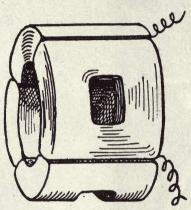
FIG. 4. DETAIL OF SCANNING COIL
