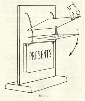
punch holes must not appear in the picture, the width of the top margin must be increased by a sufficient amount to insure that the mounting holes do not appear in the televised picture. The arrangement of guide wires shown in this drawing has been designed to maintain accurate focus of the title pickup.
