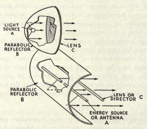
FIG. 1. PARABOLIC REFLECTORS
