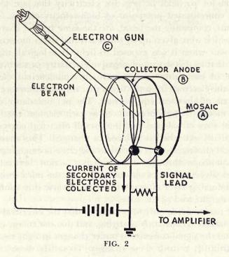
mosaic produces a series of individual electrical charges which duplicate in quantity and arrangement the lights and shadows of the scene before the lens of the camera. Light energy is thus transformed into electrical energy, but it remains for us to col-
