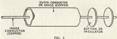
does not lend itself to bending or to use under conditions where the inner conductor does not remain in the exact electrical center of the outer tube. Flexible co-ax, which we use for interstage connections and non-rigid transmission work, such as the camera cable, is shown in Figure 6. This type, while less
