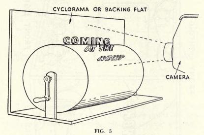
category. A simple but efficient unit is the title drum shown in Figure 5. Such a unit is excellent for work where the cast is limited in number and the credits are not extensive. It does not lend itself to extended copy.
