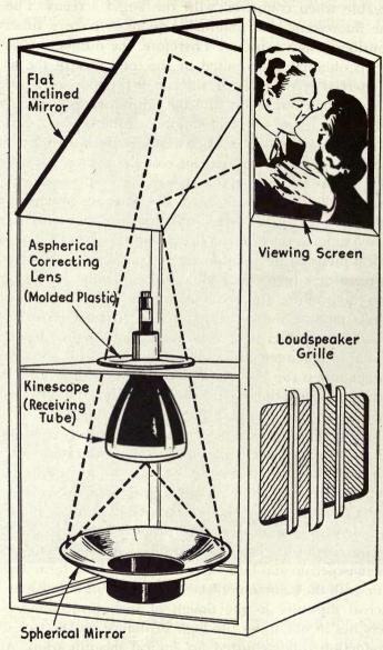
LARGE-SCREEN TELEVISION FOR THE HOME, DEVELOPED BY THE RCA LABORATORIES. Broken lines indicate the path of light beams from a single picture element on the face of the cathode-ray receiving tube to a corresponding point on the screen. A plastic lens is used to bring these light beams to a sharp focus on the screen
