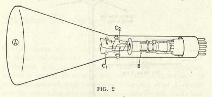
willemite salts, or an equivalent phosphor capable of fluorescing under the impact of an electronic beam.
