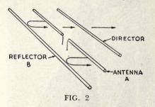
the back of the antenna to be reflected in phase with the original radiations and thus fortifying the output that would be obtained by the antenna alone. A further increase in efficiency is obtained by placing a measured rod or director antenna at a com-
