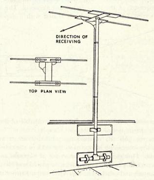
FIG. 1. DIPOLE RECEIVING ANTENNA WITH REFLECTOR
