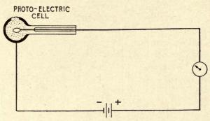
FIG. 32a.-The essentials of a photoelectric cell circuit.
