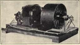
(Courtesy of Jenkins Laboratories.) FIG. 116.—Jenkins' drum-scanner. Note quartz spokes.
