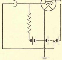
FIG. 29.—Use of a vacuum-tube amplifier in connection with a photoelectric cell.
