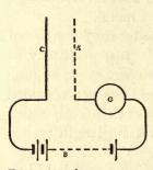
FIG. 26. — Apparatus as used by Stoletow in studying photo-emission.
