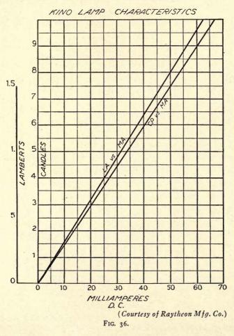
These lamps are current operated. In order to get maximum contrast between the light and shade of a picture it is necessary that their brightness change over a maximum range with current change. The lower curve, Fig. 36,
