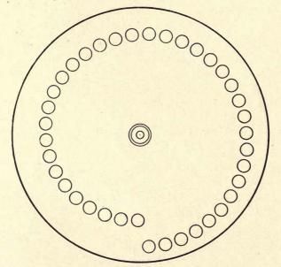
FIG. 73.—Baird lens disc showing spiral arrangement by means of which the scene is scanned.
