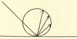
FIG. 10.—In the case of a diffusing surface reflection follows Lambert's cosine law. This is shown above where the length of arrow represents the amount of light reflected in any chosen direction.
