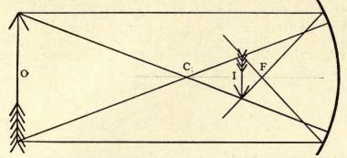
FIG. 12a.—The position of the image and its size with respect to the object when the object is beyond the center of curvature is shown above.
