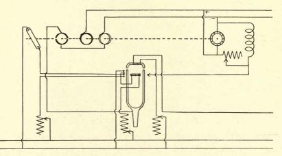
FIG. 53.—Schematic diagram of circuit used for synchronization in the Ranger system. Neon tube, at upper left, is connected to motor shaft, at upper right, and is used as a stroboscope.
