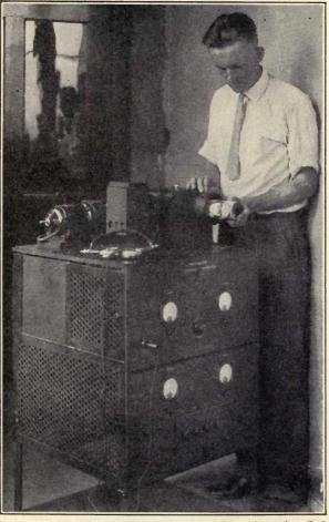
(Courtesy of the Westinghouse Electric and Manufacturing Co.) FIG. 70 b.—Westinghouse facsimile transmitter, showing photograph to be sent.
