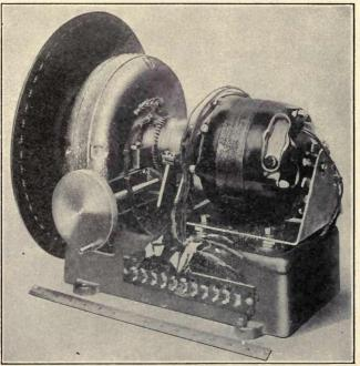
(Courtesy of the Bell Telephone Laboratories, Inc.) FIG. 109.—Mounting of scanning-disc drive as used by Bell apparatus.
