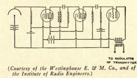
FIG. 66 .- Photo-cell amplifier of the Westinghouse facsimile transmitter.
