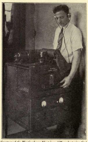
(Courtesy of the Westinghouse Electric and Manufacturing Co.) FIG. 71.—Westinghouse facsimile receiver. Note photographic dark bag over cylinder on which print is made.
