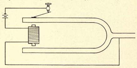
FIG. 52.-Electrically driven tuning fork.
