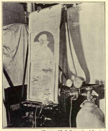
(Courtesy of Radio Corporation of America.) FIG. 62.—Enlarged reproductions made by radio picture reception apparatus of R. C. A.
