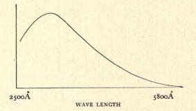
FIG. 30.—Sensitivity curve for a typical potassium hydride photo-sensitive surface. Maximum occurs in the upper ultra-violet region, about 3650Å.
