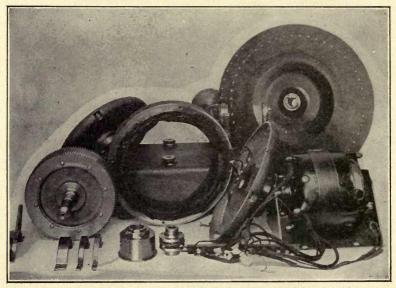
(Courtesy of the Bell Telephone Laboratories, Inc.) FIG. 108.—Assembly of scanning-disc motor used by Bell apparatus.
