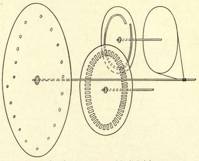
FIG. 47.-Scanning arrangement used in the Baird system.
