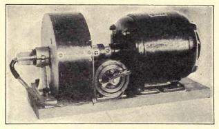
(Courtesy of Jenkins Laboratories.) FIG. 117.—Mounting of Jenkins' drum-scanner.
