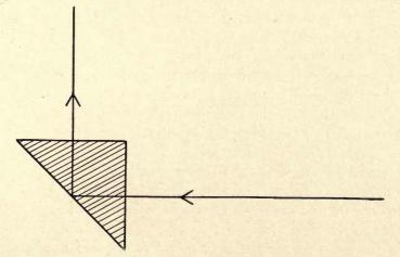
FIG. 18.—A right-angled glass prism may be used as a perfect reflector if light is allowed to strike it as shown.
