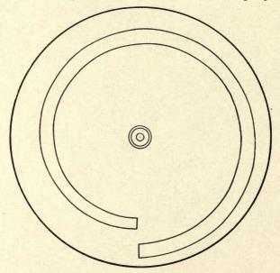
FIG. 75.—A spiral disc, just in front of the photoelectric cell, produces "finer grained" scanning.
