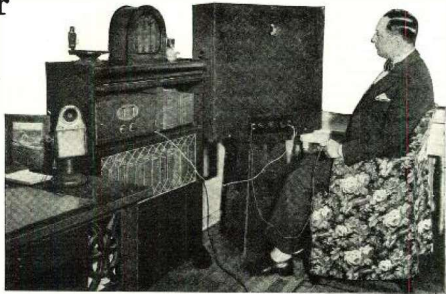
H. Gernsback, Editor of RADIO NEWS , receiving the television broadcasts from WRNY at his home in New York City, with the simple apparatus described in this article. For purposes of the test, the neon tube and loud speaker were connected in series temporarily, with successful operation simultaneously.
