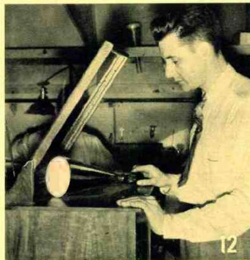
(16.) Allen B. DuMont examines a 12 in. Cathode Ray tube. This is one of the largest manufactured. They must be gingerly handled because of the constant danger of an implosion (the opposite of "explosion"). With careful construction and the shifting of the stresses to the center of the tube (See picture No. 4), this occurrence is minimized. The source of the implosion is the external air pressure of 15 lbs. to the square inch to which the tube is constantly subjected. Without the outside air pressure, C.R. tubes could be built to any size and the picture projected could be as large as the ordinary movie.
