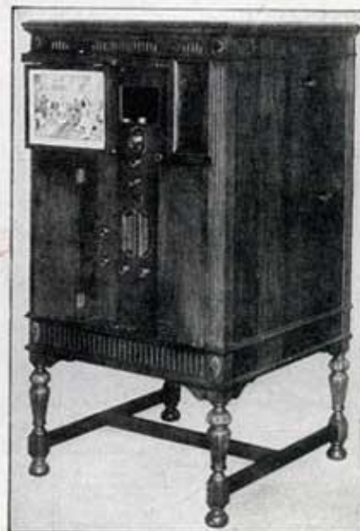
The Shortwave and Television Co.'s new double unit has an all-wave tuner with loud speaker for voice; and a short-wave television tuner, with neon lamp and scanner, behind the screen at the left. (1204)
