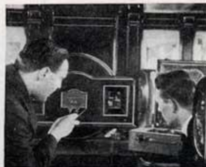
In the standard English televisor, the image is scanned vertically at the side of the disc. This is a scene on an English train.
