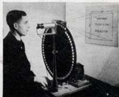
The Hartmann scanner, with its large lenses and powerful crater lamp, can throw an image three feet square on a screen. (1203)
