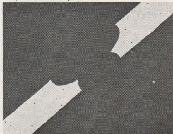
Fig. 3. Photomicrograph of a typical shadow-mask hole shows tapered hole that is produced to reduce electron scatter.
