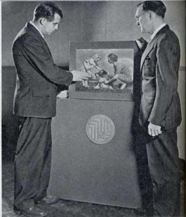
Signals corresponding to red, blue and green are picked up on three kinescopes within the receiver and projected on a 15 x 20-inch screen. Seen at left is RCA's new color slide television camera.
