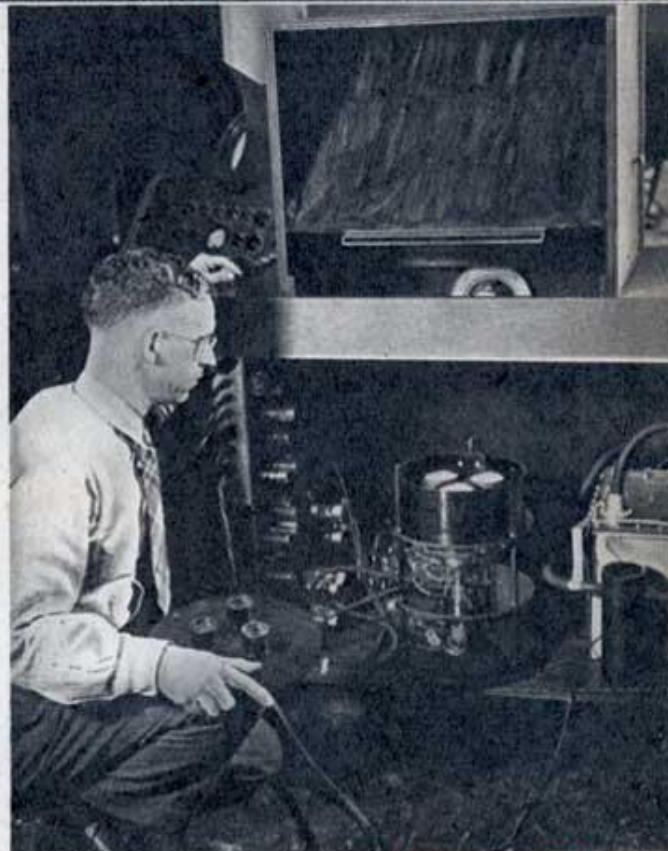
Inside the RCA receiver. At center bottom sits the "Trinoscope" projection assembly.
