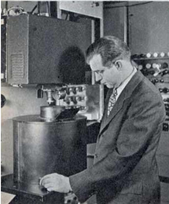
Signals corresponding to red, blue and green are picked up on three kinescopes within the receiver and projected on a 15 x 20-inch screen. Seen at left is RCA's new color slide television camera.
