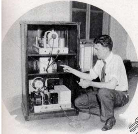
A rear view of the modern television set, showing the cathode ray tube in the upper compartment, and sound reproducer at the bottom. It is no larger than an average radio set.
