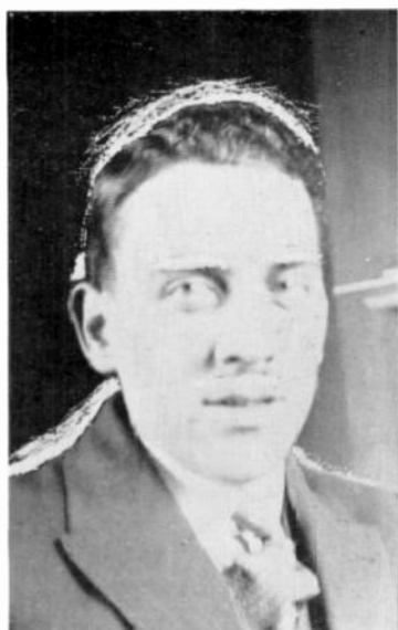
FIG. 140.—If the receiver gives undue high-frequency response, the image will be accompanied by white patches surrounding the dark sections, somewhat after the manner shown in this illustration.
