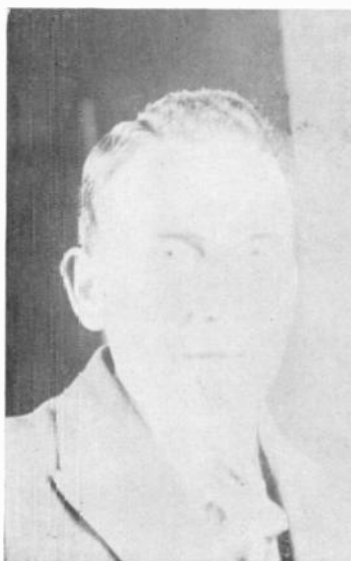
FIG. 156.—If the signals are too weak, or the lamp is too brightly illuminated from a separate source, the received image will appear like this.
