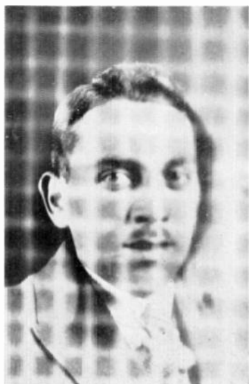
FIG. 151.—Interference such as may be caused by local oscillation will produce a chequered pattern as shown.
