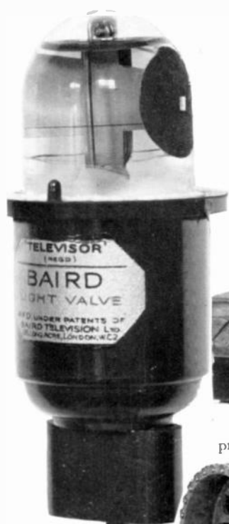
FIG. 125.—A photograph of a Baird grid cell or light valve, used in the Mirror Visor described in this book.
