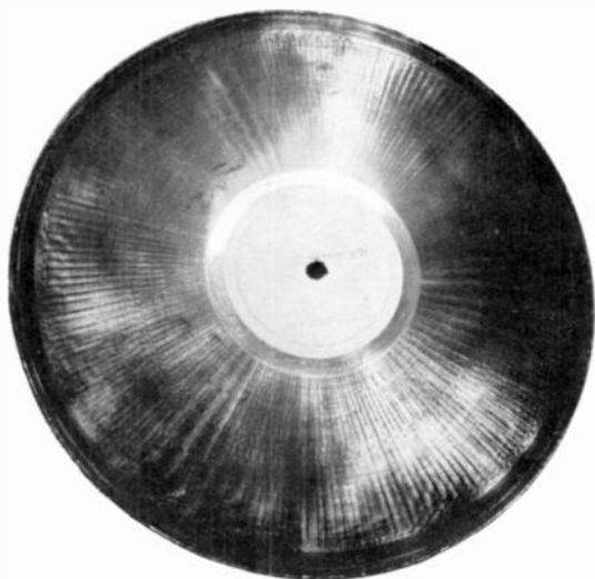
FIG. 85.—An actual phonovision disc record. When "played" on the appropriate apparatus, instead of song or music being heard, the movements of an artist can be watched in the vision apparatus.
