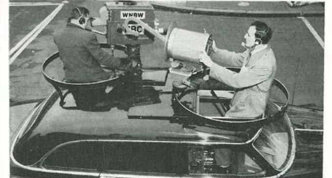
Camera and directional antenna are mounted in tank-type turrets, revolving in full circle on top of Cadillac
