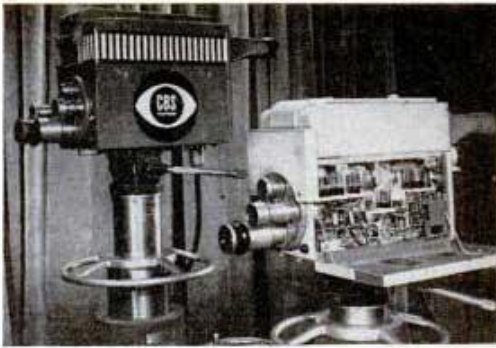
CBS color camera at right is about the same size and shape as conventional black-and-white camera at left
