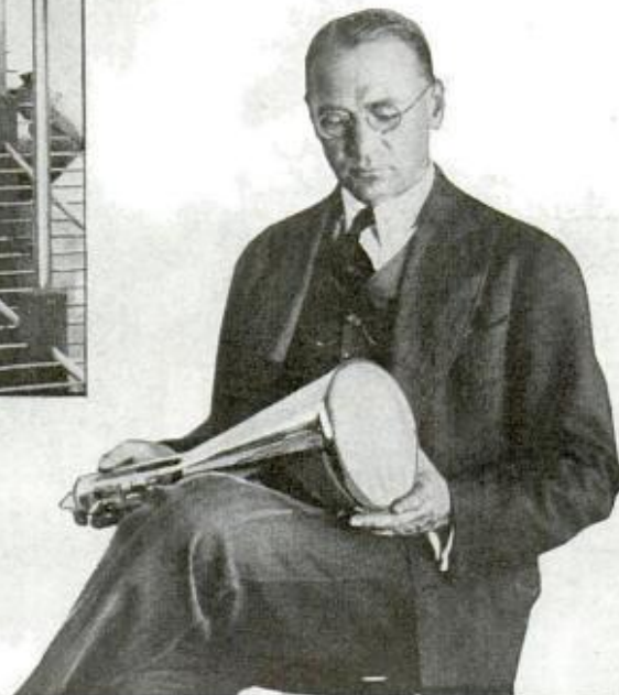
Marconi Micro-Wave Aerial System with Parabolic Reflectors; It Is Used in Experimental Work
