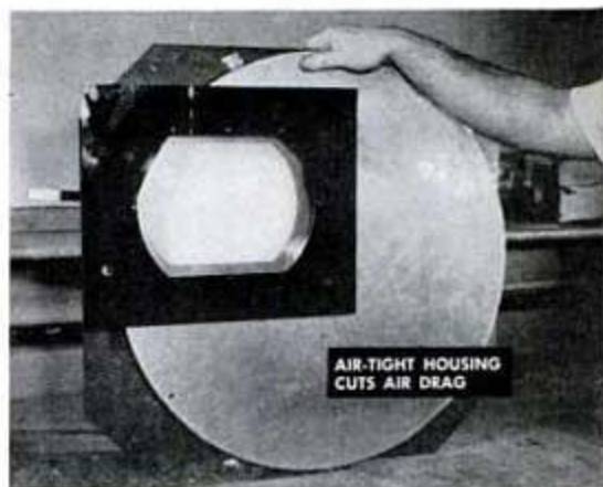
Twin wheels make it possible to see black-and-white shows without moving them aside (above). The 10-in. screen magnified to 12½-in. is as big as can be used easily with disks.
