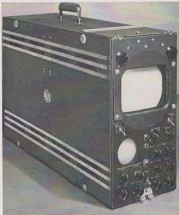
Field Camera Control Unit in carrying case.
