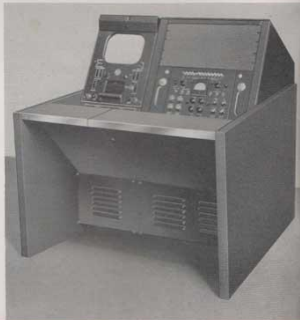
Master Monitor and Processing Amplifier mounted in new console housings. The consoles are also designed to house Camera Control Panel, Color Monitor, and other camera chain equipment.
