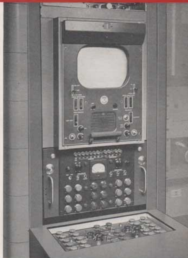
Optional rack mounting for the TK-41 control equipment may be specified. A convenient desk with top panel removed to reveal set-up controls is shown above.
