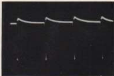
F - NEG CLAMP PULSE AT PIN 5 OF V10; 2.0 VOLTS (PEAK-TO-PEAK)
