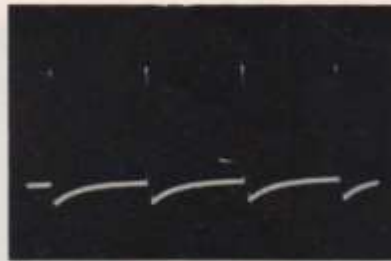
G - POS CLAMP PULSE AT PIN 7 OF V10; 2.0 VOLTS (PEAK-TO-PEAK)
