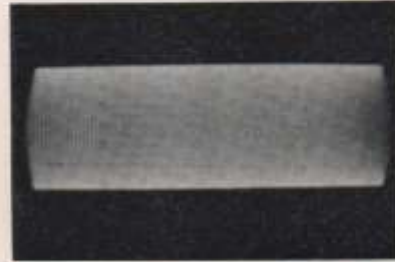
F - 3.579 MC, 90° PHASE SHIFT AT J22; 2.0 VOLTS (PEAK-TO-PEAK)
