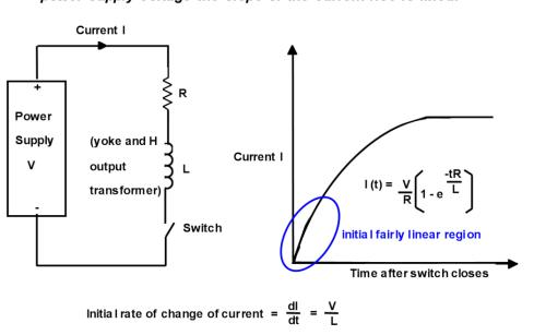
For any Yoke and Horizontal output transformer combination and power supply voltage the slope of the current rise is fixed:
