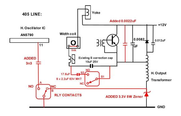
The 3.3V zener temperature was a little high at about 90 Deg C. While is rated to 200 Deg C, I felt it was better to solder it to a brass lug and screw it to the chassis to help drag heat away from the junction.
