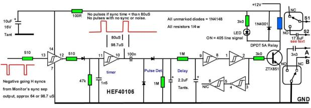
The simple detector circuit based on a Hex inverter Schmitt trigger IC is shown below:
