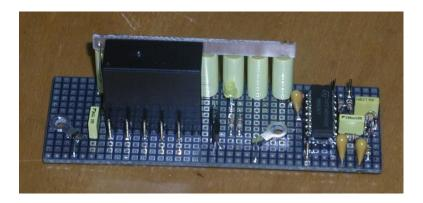
The eight 2.2uF 63V capacitors that comprise the modified S correction capacitor value for 405 line mode can be seen in a row behind the relay.
