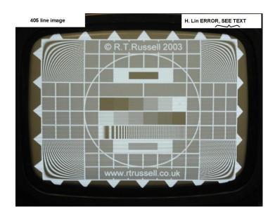
S correction cap = 10uF in 405 line mode
