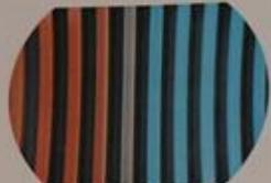
Figure 4-40 — Color Bar Pattern with  $Q$  Signal Missing
