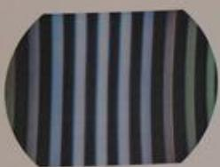
Figure 4-41 — Color Bar Pattern with  $I$  Signal Missing
