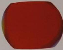
Figure 5-23—Uniform Red Raster in Center of Screen
