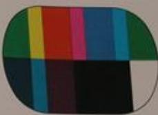
Figure 4-45 — Color Bar Pattern with Red Grid Shorted
