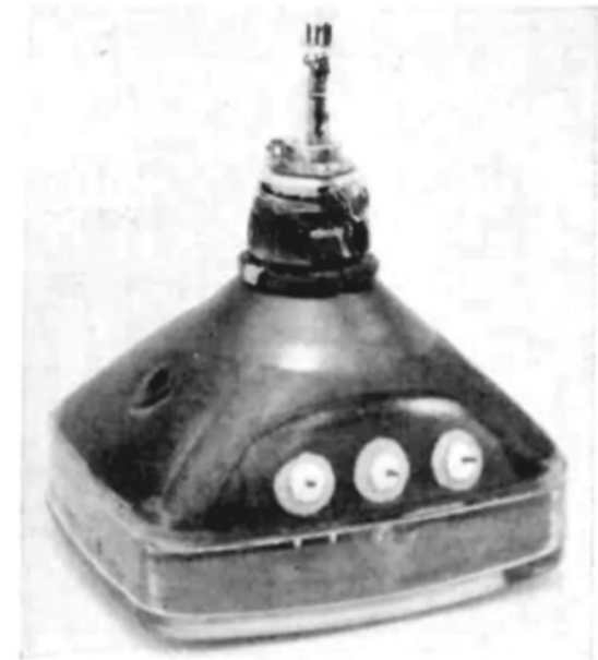
This view of the Colornetron beam-switching tube used in Japanese Yaou sets shows the three high-voltage electrode connections. The center pin is for the focusing grid, which gets 6.3 kv. The outer pins connect with the beam-switching grid, which gets 4.7 kv peak to peak.
