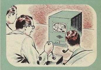
Nuclear physics involves work with dangerously radioactive materials. Operations must be performed behind radiation-proof barriers, and manipulations by remote control. Exposure of operators must be prevented at all costs. The "Utiliscope" gives the operator a clear view yet cannot transmit deadly emanations. Powerful X-ray machines used in radiation therapy also are dangerous to operators. With the "Utiliscope" on the job, all possibility of exposure is easily avoided.
