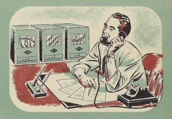
For economical scheduling and pacing of assembly in large mechanized plants, the supervisors must be able to see what is going on. The "Utiliscope" can watch feed lines and assembly conveyors at any number of remote points. Images brought right to a dispatcher's desk enable him to give direction before production delays occur. Shortages are caught before they become serious. Pile-ups are straightened out while still small. Misdirected materials are redirected.
