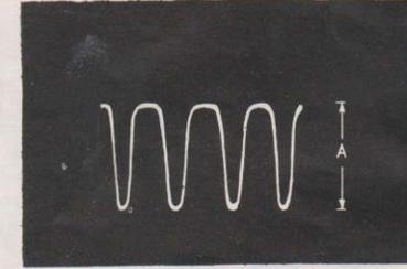
Oscillator Tube Plate Tube V23 Pin 3
