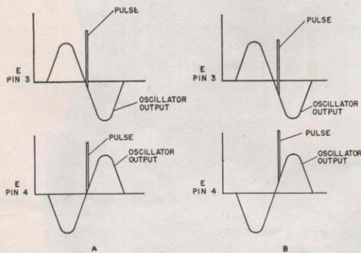
4(a) Oscillator Synchronized to Pulse Frequency      4(b) Oscillator Not Synchronized to Pulse Frequency
