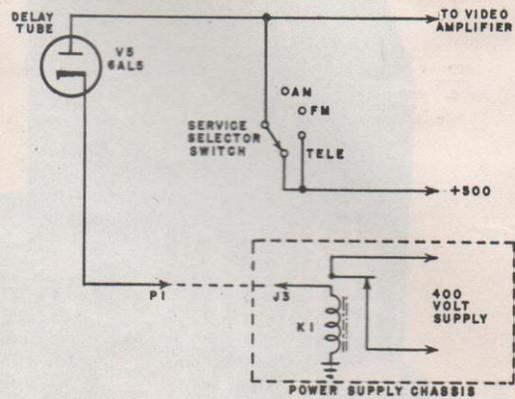
**Figure 5. Simplified Delay Tube Circuit**
