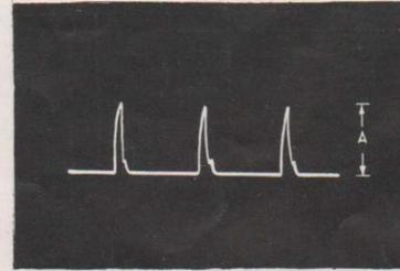
Horizontal Clipper Plate Tube V18 Pin 2
