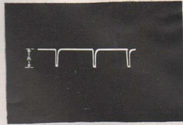
Sync Separator Plate Tube V15 Pin 2
