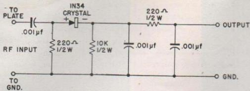
Figure 6B. Probe Detector Circuit
