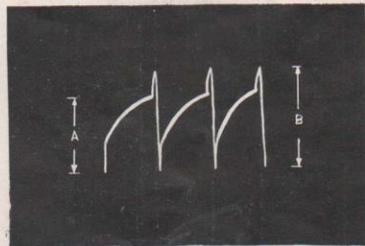
Vertical Saw Gen Grid Tube V16 Pin 4
