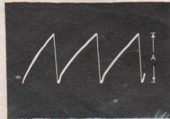
Horizontal Saw Gen Plate Tube V18 Pin 5
