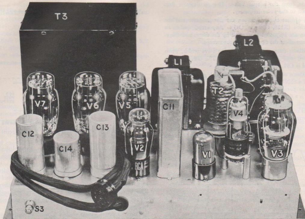
Figure 3. Power Supply Chassis Layout (RA-102)
