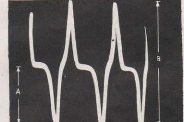
Horizontal Saw Gen Grid Tube V18 Pin 4
