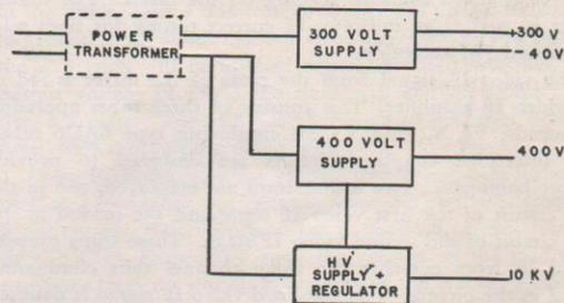
Figure 1B. Block Diagram of Power Supply Chassis
