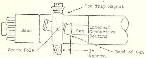
With the base end of the gun pointing up as shown, slide the magnet over the neck. The north pole should be to the left adjacent to pin #12 and the south pole to the right adjacent to pin #6. The magnet should be placed about 4" in back of the bend in the gun for the first adjustment.
