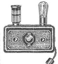
The Bair Shortwave Converter has been designed as an attachment to practically any type of radio broadcast receiver to make it adaptable to tune in on shortwaves. Shortwave reception differs radically from reception on the regular broadcast bands in the fact that
