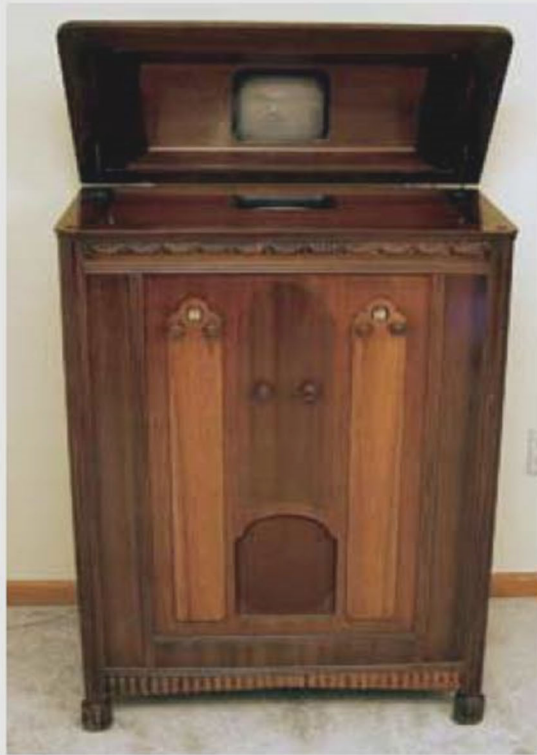
Fig. 48. RCA prototype CRT television receiver used in a field test, 1932. (Darryl Hock collection)
