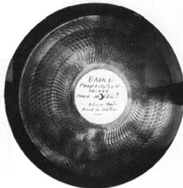
Fig. 1. The Phonovision discs all resemble 25cm (10in) diameter single-sided 78rev/min 'shellac' audio discs. A distinguishing feature is the radial structure.
