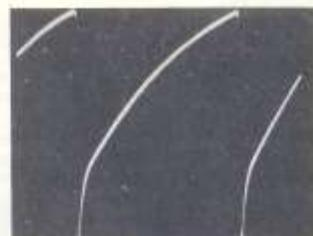
(9) Vertical oscillator plate (pin 6 of 6DR7, 55), 100 volts or vertical output grid (pin 3 of 6DR7, 55), 110 volts, 60 c.p.s.
