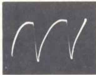
(19) Horizontal output grid (pin 5 of 6DQ6A, S11) or horizontal oscillator buffer plate (pin 6 of 6CG7, S8), 153 volts, 15,750 c.p.s.
