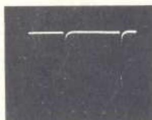
(7) Sync separator output, plate of 6AW8A (pin 3 of 59) or terminals L14 or L31, 44 volts, 60 c.p.s.
