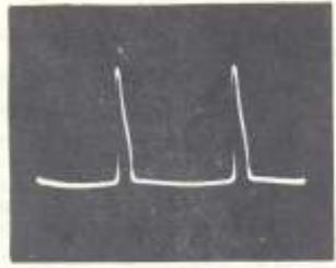
(15) Horizontal oscillator cathode (pins 3 and 8 of 6CG7, S8), 17 volts, 15,750 c.p.s.
