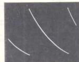
(11) Vertical oscillator cathode (pin # of 6DR7, 55), 14.5 volts, 60 c.p.s.
