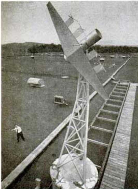
MINIATURE PLANE MOCK-UP helps determine how far transmitting antenna must project down from fuselage, so that the plane's underbody won't reflect and garble signals during turns.
