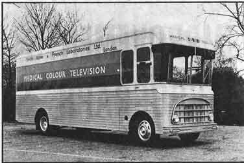
The complete colour TV system is housed in this van, the interior of which is divided into two compartments and driver's cabin. The van weighs 8 tons fully loaded, 2 tons being accounted for by the TV equipment.
