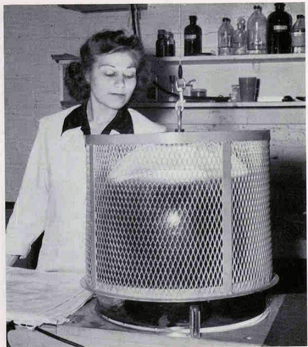
10. The aluminizing procedure consists of placing the glass bowl—inner side down—in a bell jar which is then evacuated. In the jar are two aluminum filaments from which aluminum is evaporated by heating to incandescence. The aluminum vapor which is driven off condenses on the under side of the glass.
