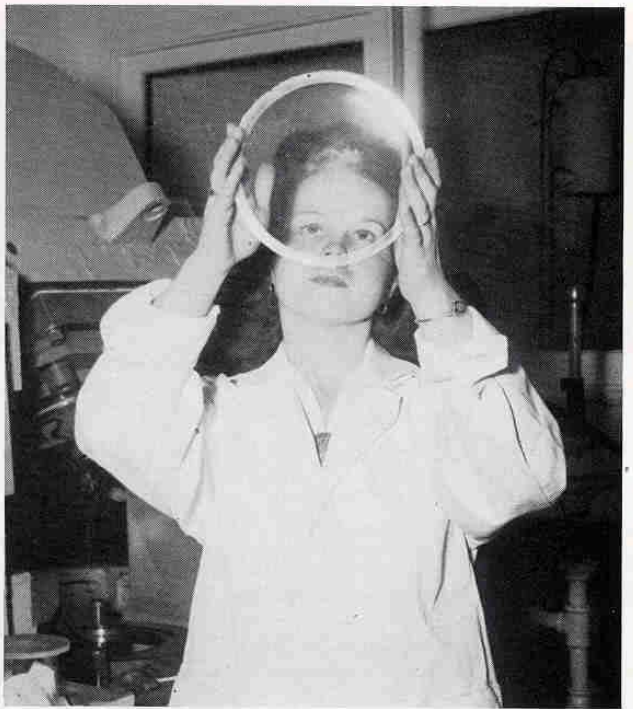
8. Lenses molded in this way have excellent optical properties. They have slightly better light transmission than glass and slightly less light scattering—both of which are, of course, advantageous. They do not have the surface hardness of glass, but in tests have stood up well without any special care.
