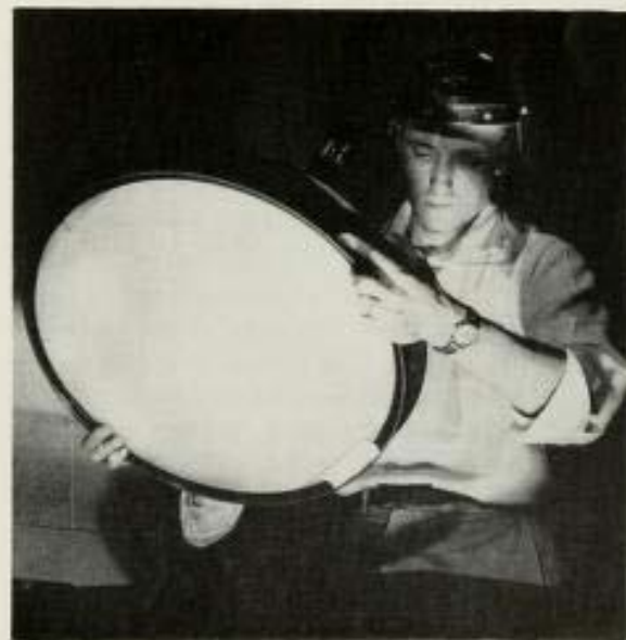
Skilled hands insert RCA 21-inch color picture tube in a receiver on the production line.
