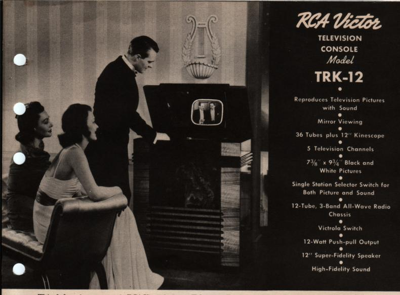
This de luxe instrument is RCA Victor's finest Television Receiver. Not only does it reproduce pictures in unusually fine detail and of ample size, but it also includes a 12-tube, high-fidelity, 3-band, all-wave radio. A unique feature is the indirect viewing of the image. This feature in conjunction with the large image size makes it possible for a large group of people to view a program with ease. It also makes possible a more compact cabinet design.
