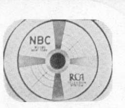
Figure 3-INCORRECT FOCUS To correct-Adjust Facusing Control for shurpest image
