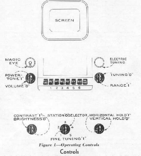
Immediately beneath the Television picture screen is the Radio dial with Magic Eye Electric Tuning Indicator, a row of push buttons and two dual Control Knobs. Below these is a row of three more dual Control Knobs. The dual knob at the left of the push buttons is an all purpose control being used for Television and Radio reproductions.
