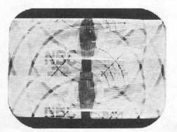
Figure 7—INCORRECT VERTICAL HOLD To correct—Adjust Vertical Hold Control until picture "locks in"
